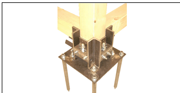
Figure 13: Photo of the foundation prototype realized in 1:1 scale
