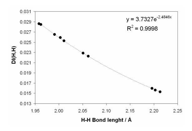
**Fig. 2** Correlation between QTAIM delocalization index (DI(H,H)) and the internuclear separation of hydrogen atoms linked by a bond path.
